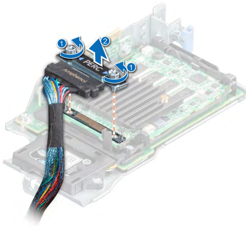
Figure 28. Disconnecting the cable from internal PERC card
